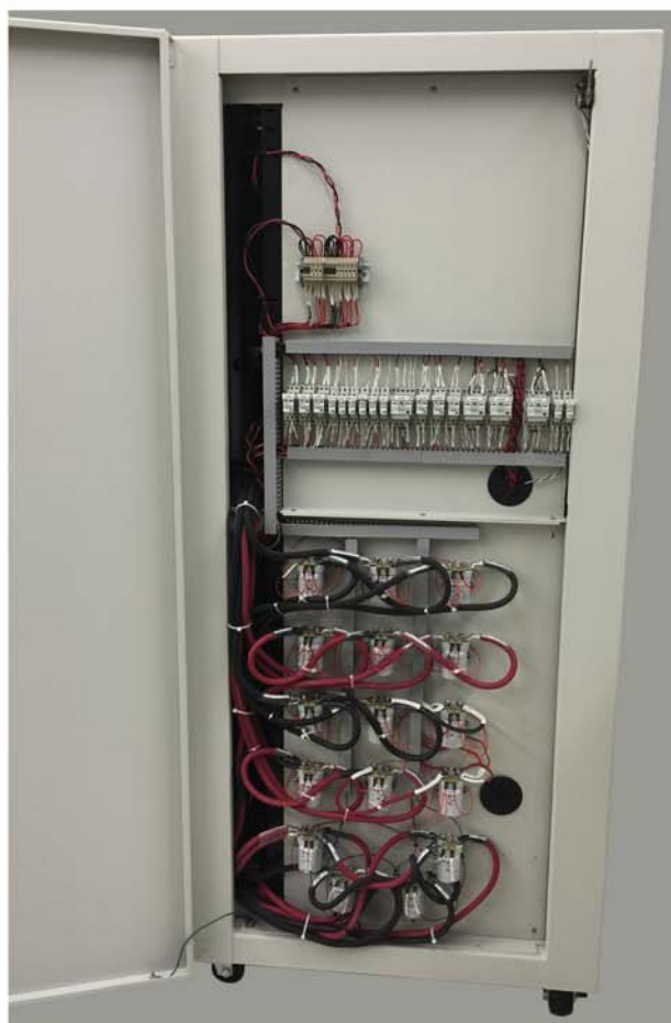
Left-Side Cabinet Extension Open showing High Power Relays, DIN Rail Relays, Terminal Blocks, etc.
