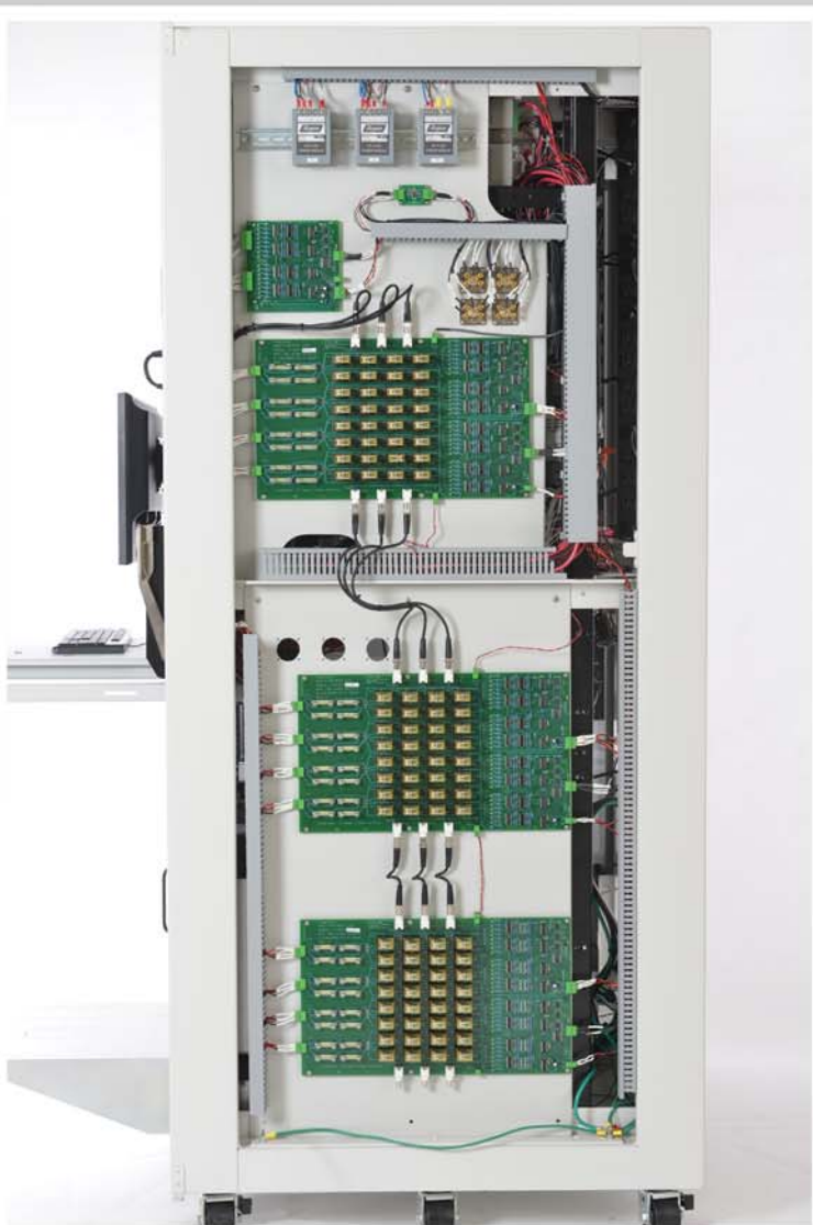
Side view with Left Extension Open allowing easy access to all of the Switching Matrix Cards, HF Relays, Power Supplies, Relay Drivers etc
